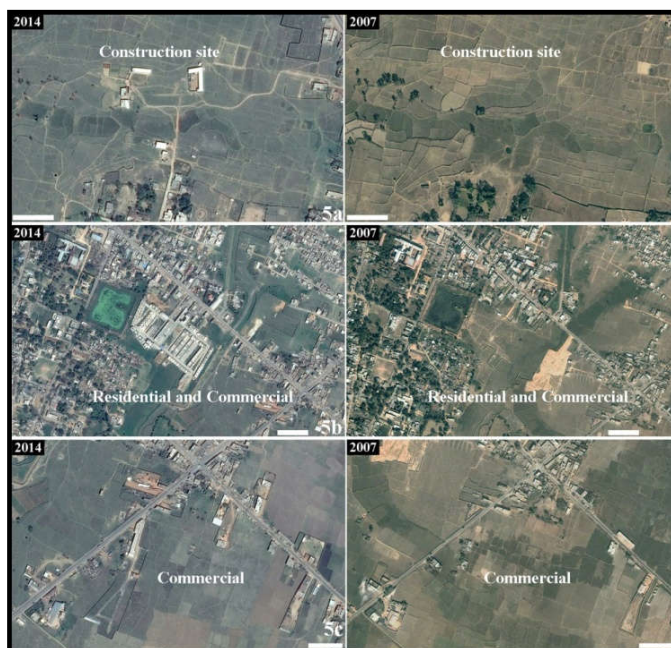
Figure no. (5a - 5c): Zoomed-in details of the sites where urbanization is inferred from Figures no. 3 and 4. Left panel is Google Earth product of 2014 and right panel is of 2007. The type of urbanization is inferred from the figures and mentioned for clarity. Scale bar is of 50 meter in all the images. The spatial locations of these figures are displayed in Figures no.3 and 4 for reference.
