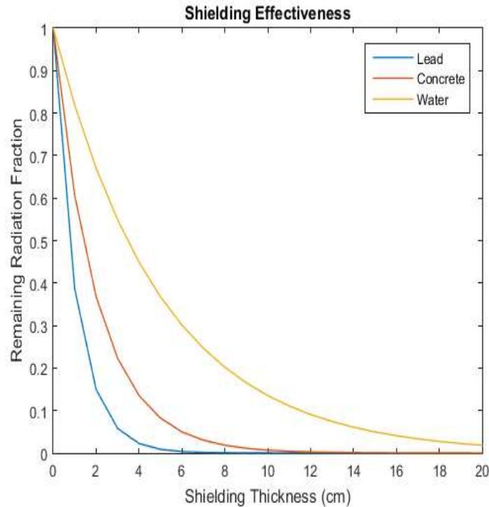
**Figure 4: Shielding Effectiveness Curve**
